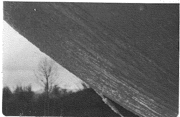
Fig. 4. Ice collects on rigging and aerostat surface
